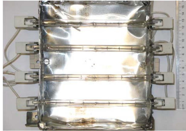
Fig.3. Photo of experimental infrared heater for welding of plastic details with halogen lamps. Nominal power 4 kW (at 230V).
